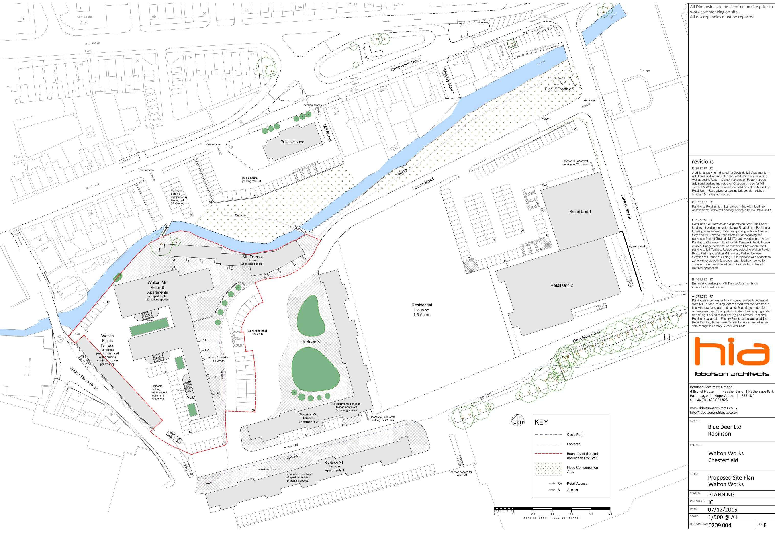
Additional parking indicated for Goytside Mill Apartments 1; additional parking indicated for Retail Unit 1 & 2; retaining
